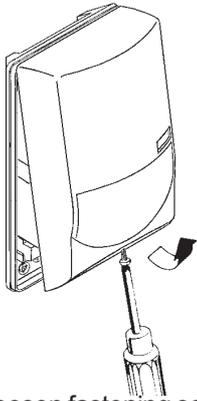
Loosen fastening screw and remove cover.
