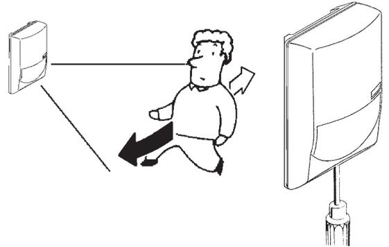
Conduct walktest and make adjustments. (Section 6) Fit cover using fastening screw.
