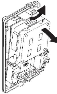
Release hook at top of unit. Remove P.C.B. unit from base.
