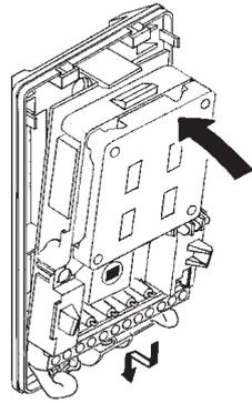
Fix P.C.B. unit into base. Supply power. Allow 30 sec to warm up.
