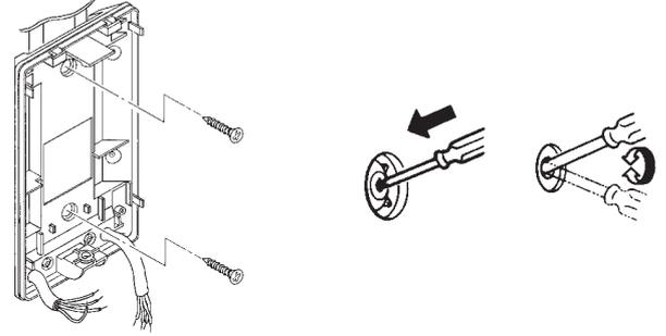
Lead in wires through knockouts along the wiring guide on the rear side of base. Mount base with supplied screws. When small animal immunity is required, refer to Section 6-E. When using a bracket, check matching knockout position before opening mounting hole.
