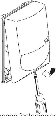
Loosen fastening screw and remove cover.
