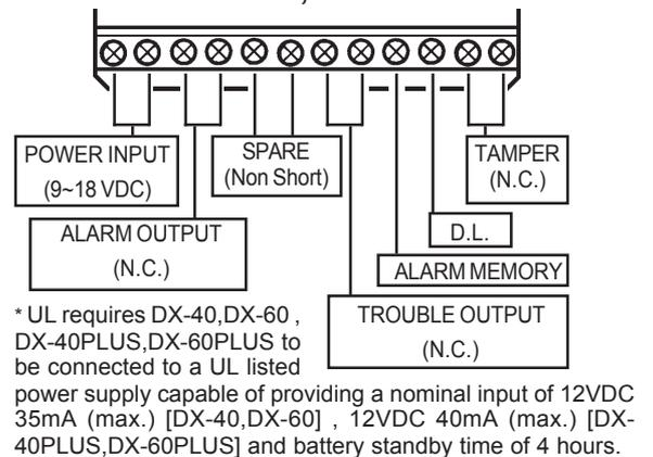
\* The equipment shall be installed in accordance with the National Electrical Code, NFPA 70.
